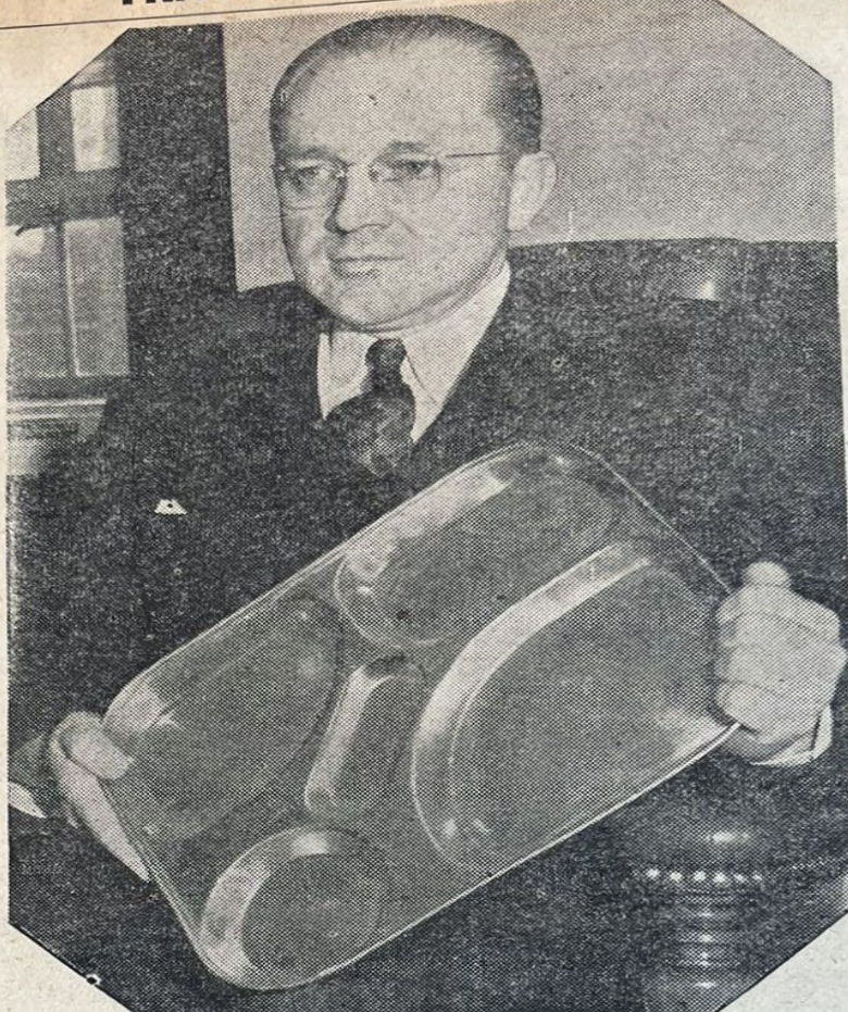
Clinton T. Duffy, Warden of San Quentin, holds one of the four-compartment trays now being manufactured at the prison. Made from soft-drawn iron, the trays are being turned out at the rate of five per minute on the 500-ton
